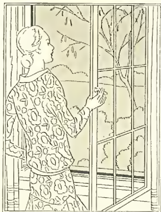
These casements (above) swing inward - - screens are outside and need not be moved except for storage in winter.
